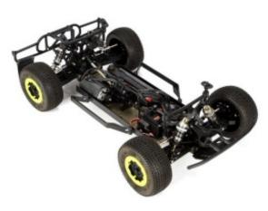
Quality RC cars or 'remoted controlled cars' are usually controlled with classic servo signals. The steering as well as the speed unit are controlled with servo signals what makes it possible to drive such an RC car with our Brainbox.
